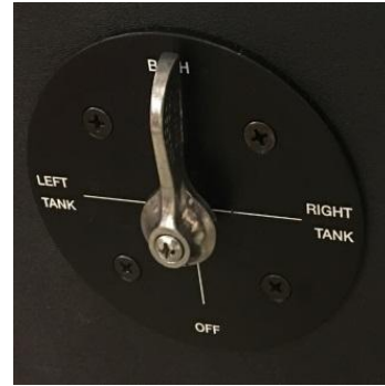
Image 62: Switch Panel 1 Fuel Selector
