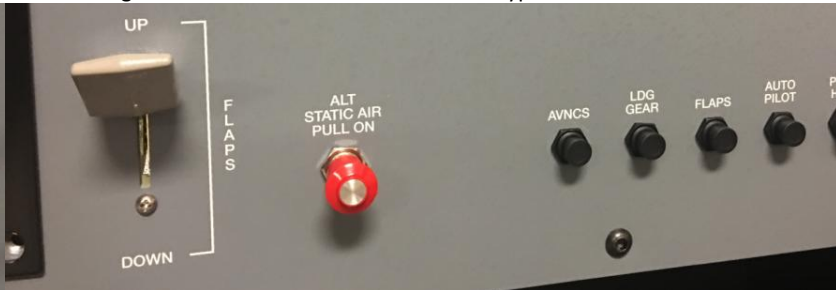
Image 46: Right Side of Lower Switch Panel Type 1, 2, & 3*
