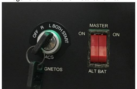
Image 47: Switch Panel 1 Starter Switch*
