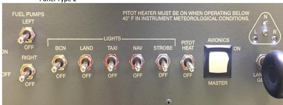
Image 59: Center of Lower Switch Panel Type 1, 2, & 3
