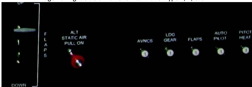
Image 48: Right Side of Lower Switch Panel Type 1, 2, & 3*
