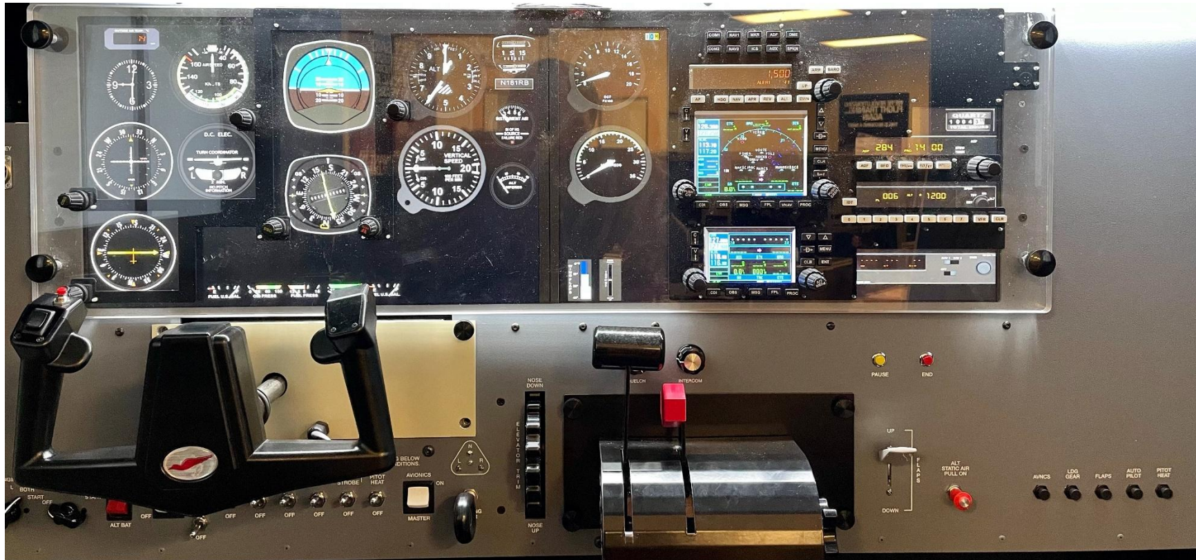
Image 25: Traditional 6-pack Instrument Panel Configuration (Example with Center Yoke and T-M Lever Throttle)
