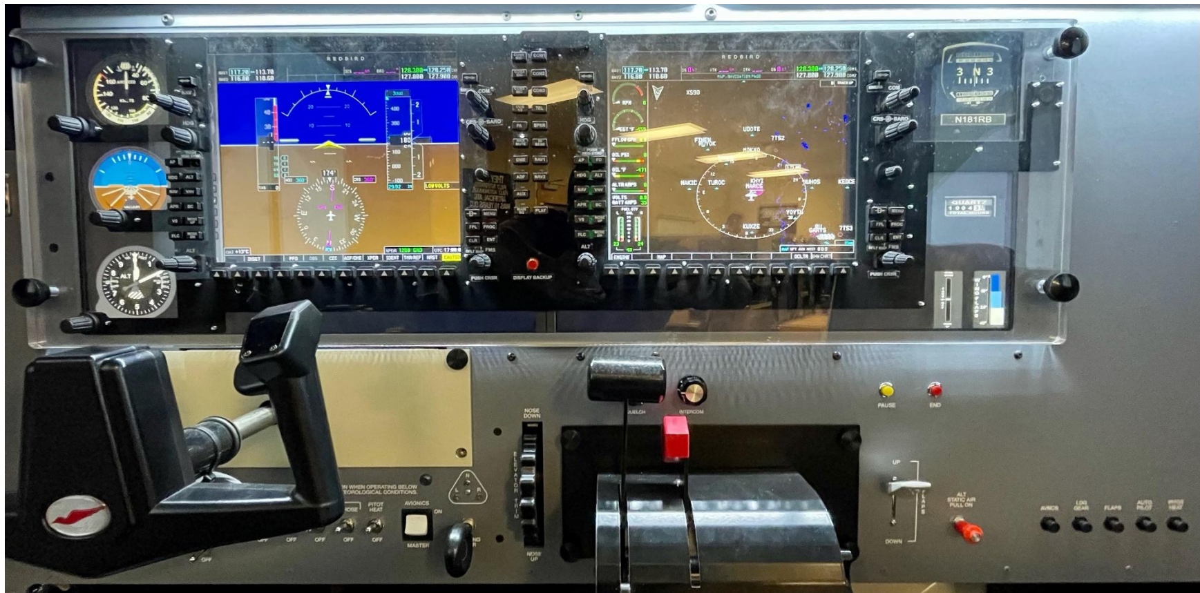
Image 26: Glass Panel Instrument Configuration (Example with Center Yoke and T-M Lever Throttle)
