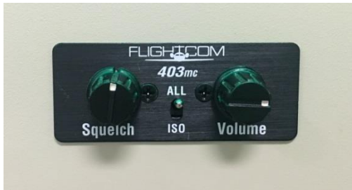
Image 52: COM Volume/Squelch Adjustments*
