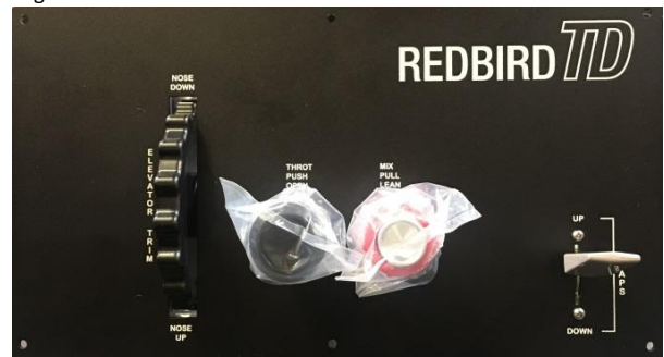
Figure 11: TD Throttle Quadrant (T-P), Trim, Flap Handle
