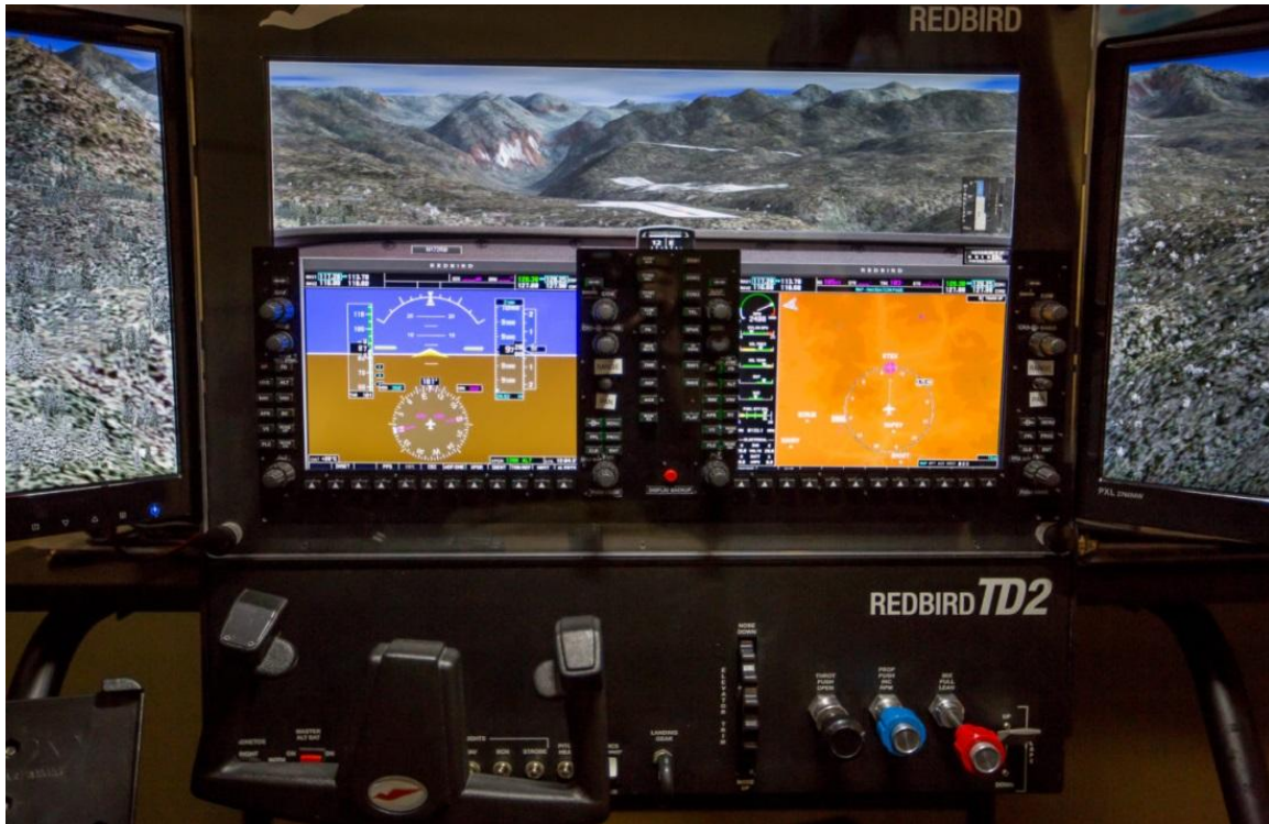
Figure 14: TD2 - Glass Panel General Overview (Shown with optional Redbird Horizon expanded visuals)
