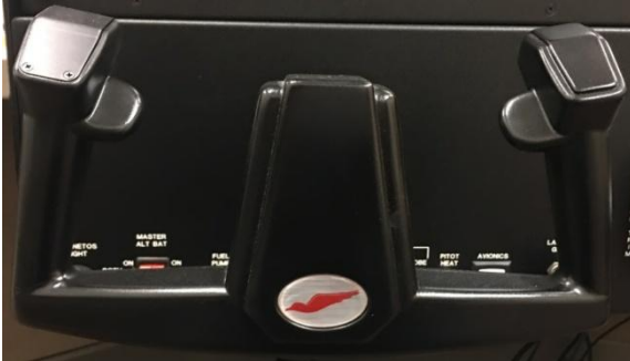
Figure 6: Control Yoke (Legacy)
