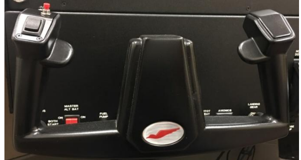
Figure 7: Control Yoke w/ E-Trim, AP, PTT Switches
