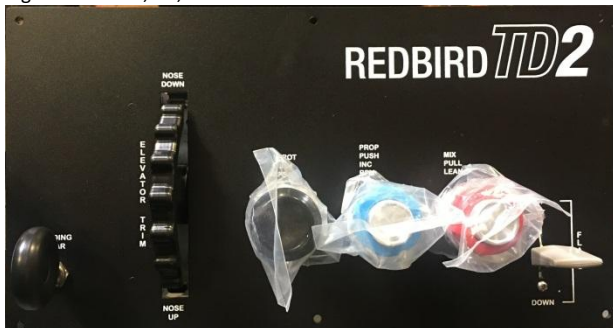
Figure 10: TD2 Throttle Quadrant (T-P-M), Trim, Gear Handle, Flap Handle
