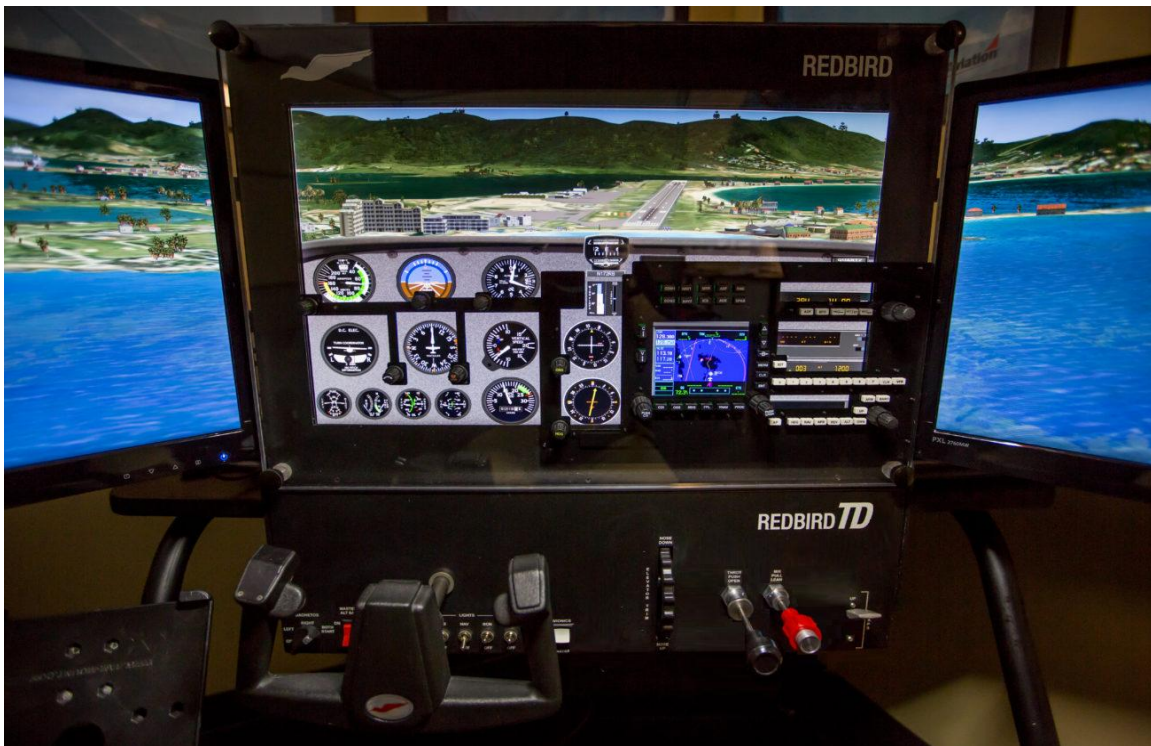
Figure 17: TD – Analog Panel General Overview (Shown with optional Redbird Horizon expanded visuals)
