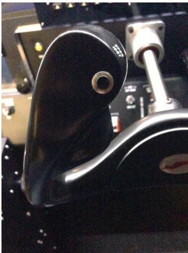
Image 12: Co-Pilot Yoke Switches – Left
