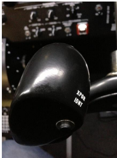
Image 13: Co-Pilot Yoke Switches – Left
