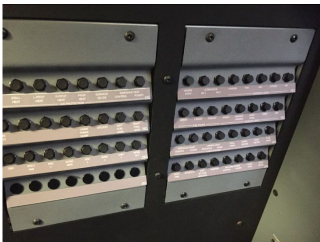
Image 14: Pilot Circuit Breaker Panel
