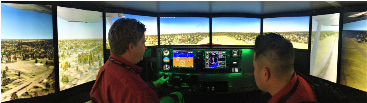
Image 26: Visual Displays – Type 4 (27” Display Monitors)
