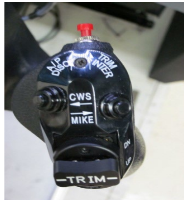
Image 7: Co-Pilot Yoke Switches – Right
