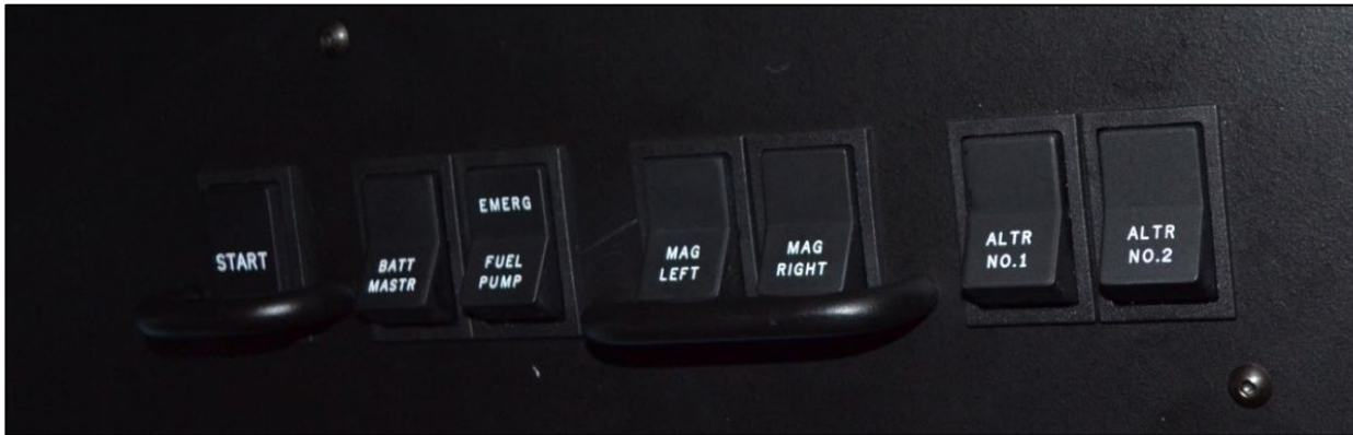
Image 17: Overhead Switch Panel (Pilot)
