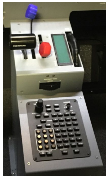
Image 9: MRG Throttle Quadrant / FMS Keypad
