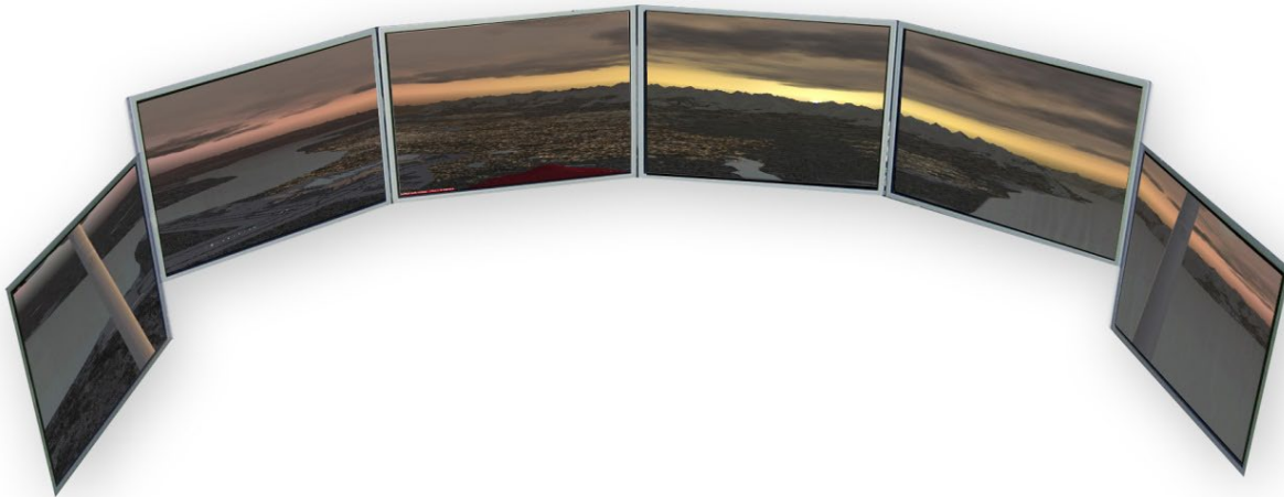
Image 23: Visual Displays – Type 1 (22" Display Monitors)
