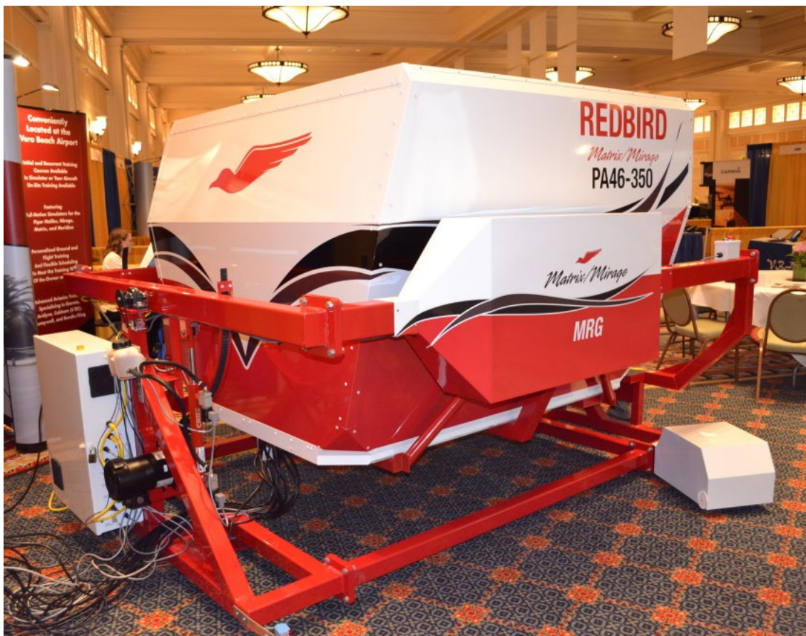
Image 22: Motion Platform and Cockpit Enclosure
