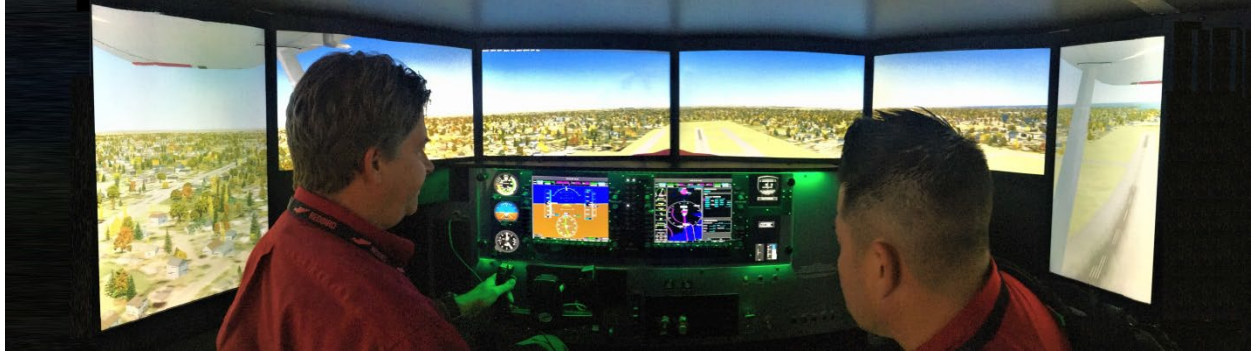
Image 25: Visual Displays – Type 3 (27” Display Monitors)
