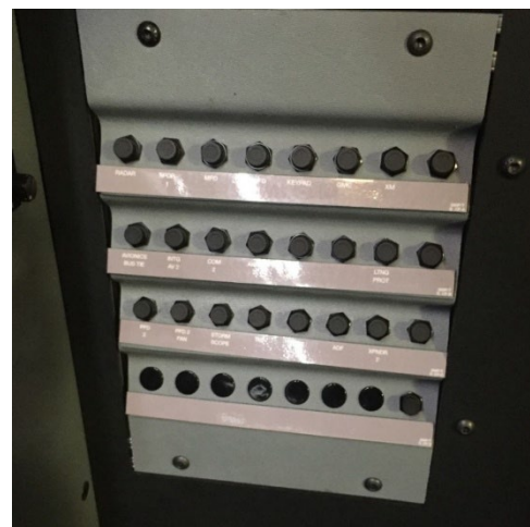
Image 15: Co-Pilot Circuit Breaker Panel
