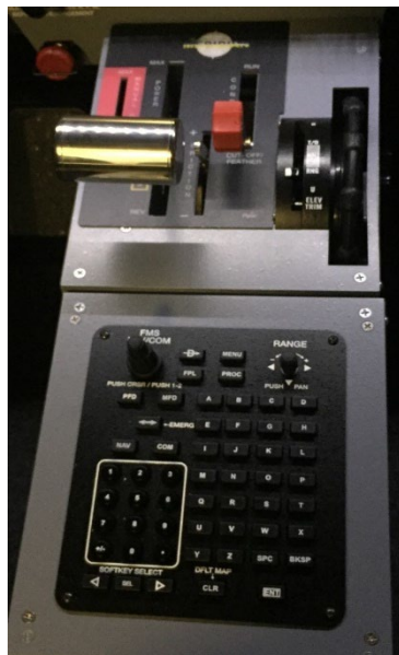
Image 8: MDN Throttle Quadrant / FMS Keypad
