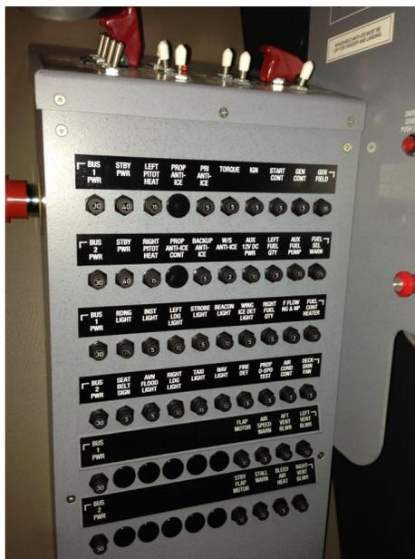
Image 18 Circuit Breaker Panel Pilots Side
