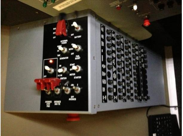
Image 20 Circuit Breaker Panel and Left Switch Panel
