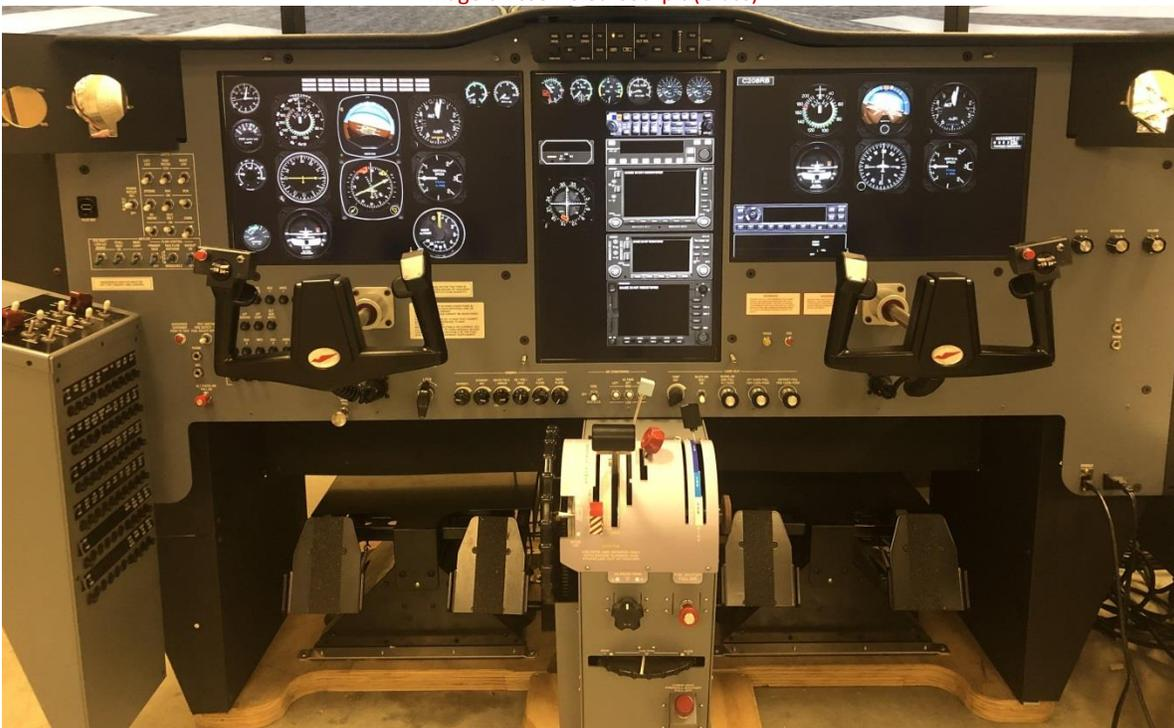
Image 7 Assembled Cockpit (Analog)
