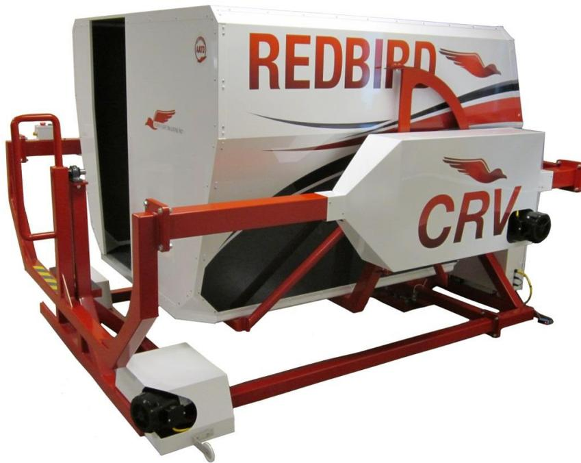
Image 26: Motion Platform and Cockpit Enclosure
