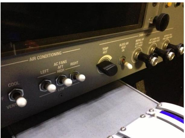
Image 24 Lower Switch Panel Co-Pilots Side
