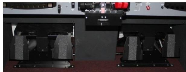
Image 25 Rudder Pedals Pilot and Co-Pilot
