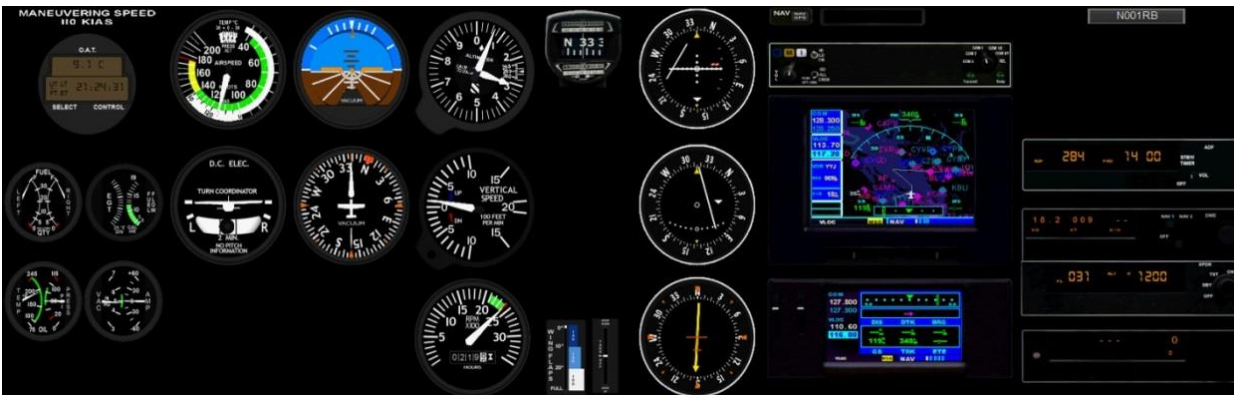
Image 5.12: Traditional 6-pack Instrument Panel Configuration (Example)
