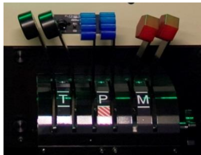
Image 3.5: Twin Engine Throttle Quadrant – Type 1
