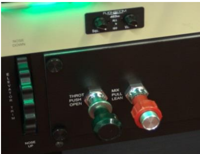
Image 3.1: Single Engine Vernier Throttle Quadrant
