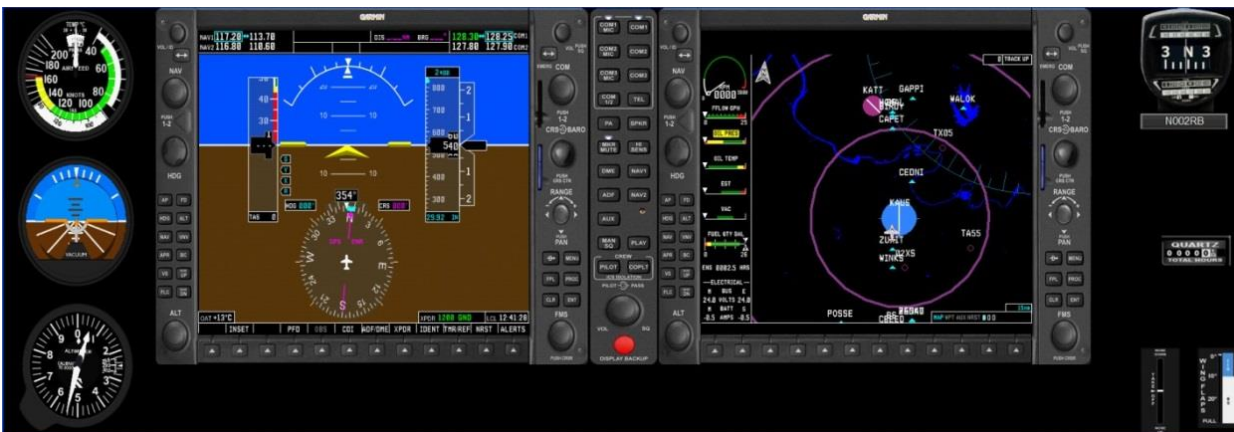
Image 5.13: Glass Panel Instrument Configuration (Example)
