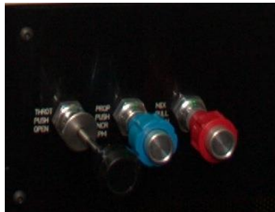
Image 3.2: Single Engine Complex Vernier Throttle Quadrant
