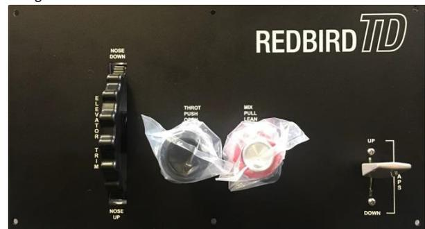
Figure 11: TD Throttle Quadrant (T-P), Trim, Flap Handle
