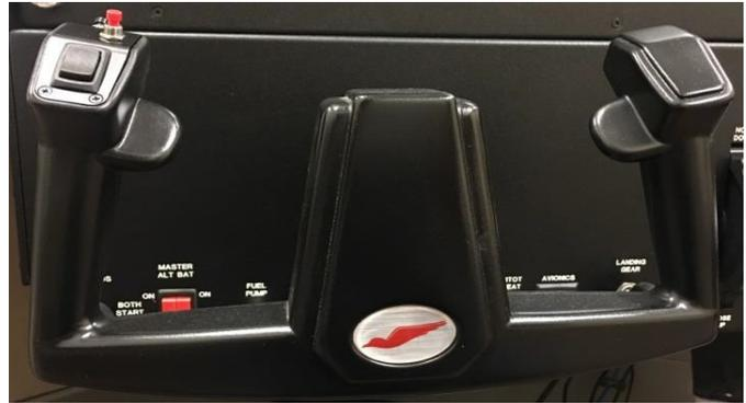
Figure 7: Control Yoke w/ E-Trim, AP, PTT Switches
