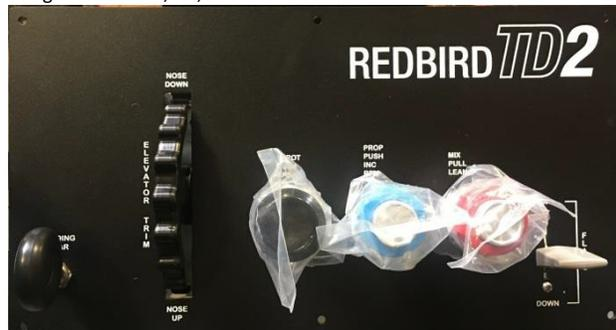
Figure 10: TD2 Throttle Quadrant (T-P-M), Trim, Gear Handle, Flap Handle
